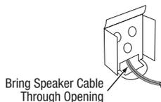
4. Thread the speaker cable through the arc-shaped opening on the top of the mounting bracket, not the screw hole.
