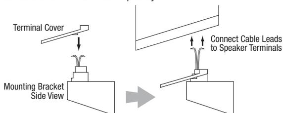
7. Fit the terminal cover into the opening on the underside of the speaker so that it is flush against the speaker and covers the terminals. Insert the supplied long bracket bolt up through the bottom of the bracket and terminal cover, and screw it into the threaded insert on the underside of the speaker. The bolt should be snug but not so tight as to prevent the speaker from pivoting on the bracket.
