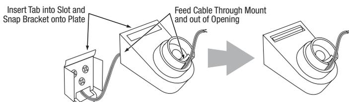
6. Fit the terminal cover onto the bracket as shown in the illustration below, then connect the speaker leads to the terminals on the underside of the speaker. Remember to observe the correct polarity.
