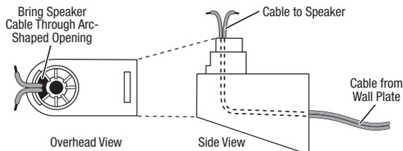
5. Attach the mounting bracket to the wall plate by inserting the tab at the top of the attachment plate into the slot on top of the bracket and snapping the bracket onto the attachment plate.
